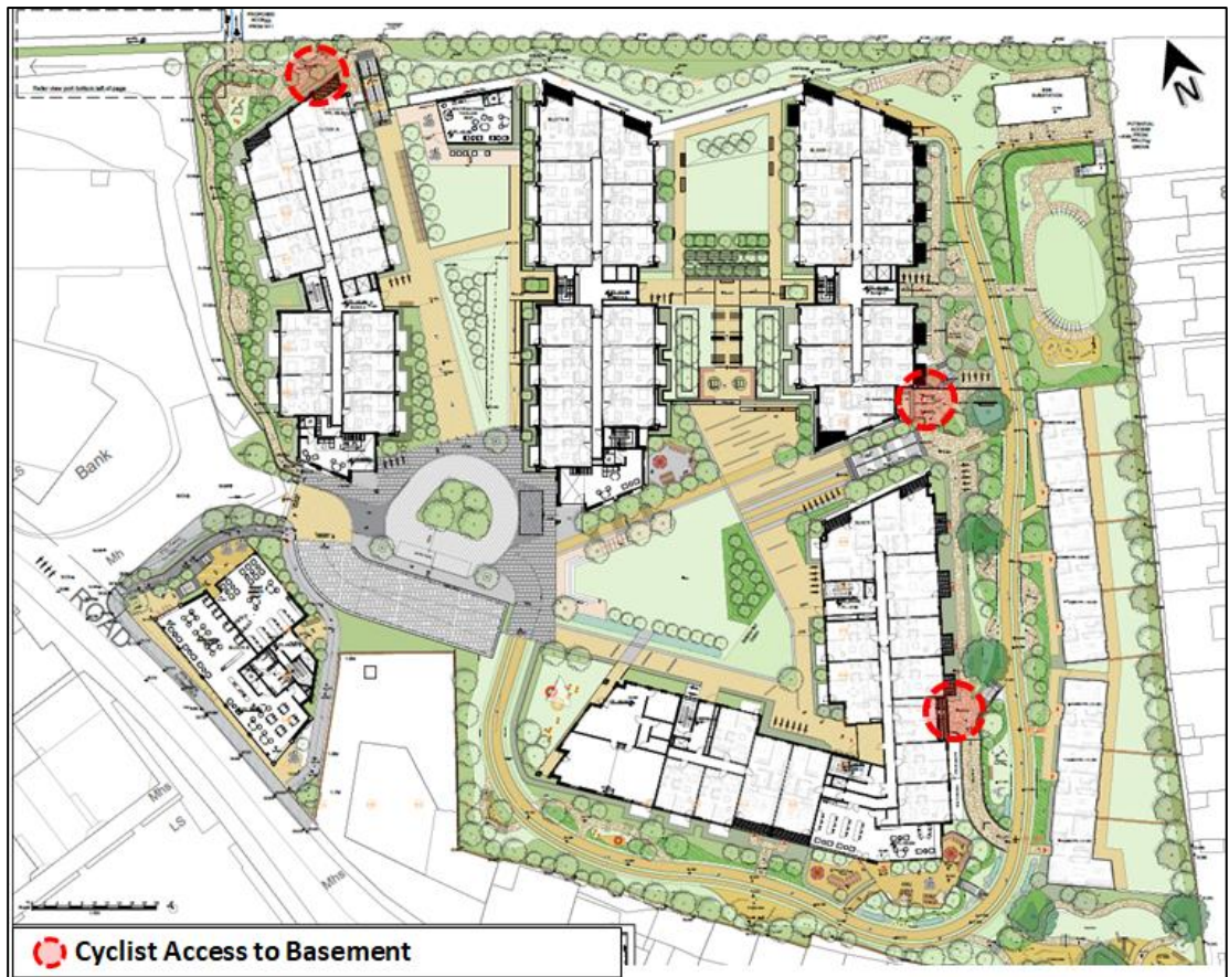
Figure 2.4: Cyclist Access points to the Basement (Source: Henry J Lyons)
